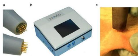
Fig. 2. Skin electroporation procedure. (a) Surface EP device. Photo shows electrode configuration. (b) ELGEN pulse generator which is tethered to the surface EP device and delivers the electrical pulses. (c) Positioning of the surface EP device on guinea pig skin.
